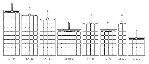
SP series is at the the top of the range, thanks to the use of selected SunPower™ monocrystalline silicon cells, reaching a record 24% conversion of sunlight into electricity and with a pleasant appearance thanks to the electrical contacts hidden on the back. SunPower™ cells represent the most advanced technology on the market, and make the SP Solbian panels the highest-efficiency flexible panels.
